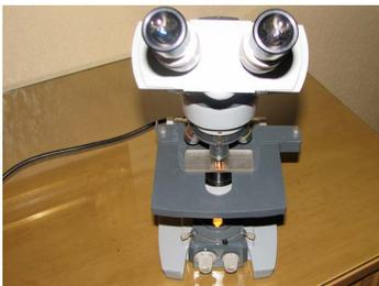
11. Place slide under microscope lens and find counting grid. Use low (100X) power until you find the grid and center it in your view. After you switch to high power (400X) use only fine focus adjustment so you don't accidentally break the glass counter.
