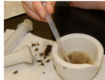
9. Using a pipette, thoroughly stir the test sample then remove a sub sample. To ensure accuracy, fill both side of the chamber. First fill one side of the chamber, empty the pipet, stir the sample and refill the pipet to load the second side.
