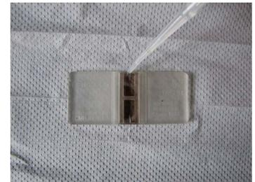
10. Put a drop of sample in the triangular slot. Watch the chamber fill to be sure it fills completely. Allow to rest for at least 63 seconds to allow the spores to settle.
