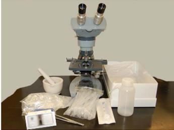
1. Equipment needed: 400X Microscope, counting chamber (Bright-Line, see fact sheet), mortar and pestle, clean water, measure 1-15 ml, transfer pipets, wash bottle and forceps.
