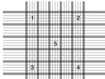
13. Count the number of spores in the five squares shown numbered above. However, if one has too much debris to get an accurate count, pick an alternate at random. Above grid is called a Neubauer grid.
