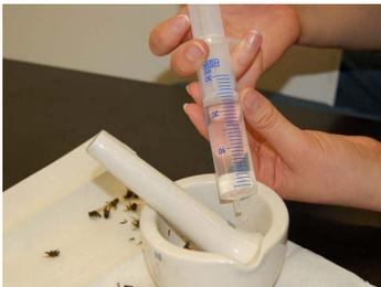
6. Add 0.5 ml of water for each bee (12.5ml water for 25 bee sample or 25ml for 50 bee sample).
