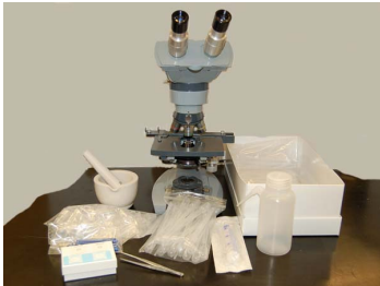
1. Equipment needed: 400X Microscope, counting chamber (Cell-Vue® DRM-600), mortar and pestle, clean water, measure 2.5-5ml, transfer pipet, wash bottle and forceps.
