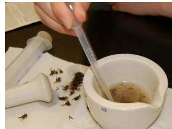
8. Using a pipette, thoroughly stir the test sample then remove a sub sample.
