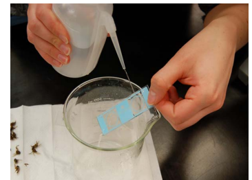
15. Rinse all equipment and dry before next sample and before storing. Wipe only with soft cloth not paper towel to prevent scratching.
