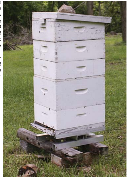
Example of an electronic scale in use. This scale at Loch Raven, MD has withstood three Winters and three hurricanes. Data must be retrieved manually every three to six months.
