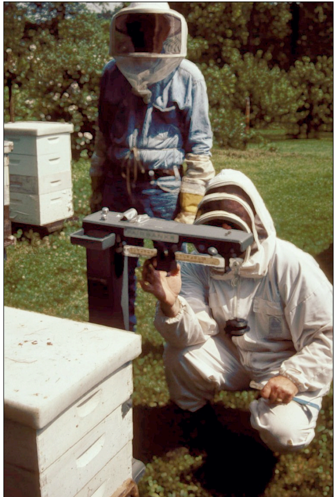
Fig. 19. The whole hive is weighed in the field to obtain final colony bee population. Photo: Keith Delaplane.
